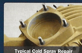
Typical Cold Spray Repair
